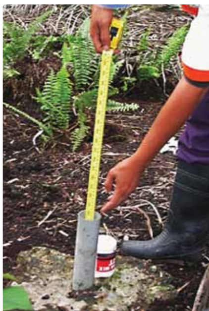
Figure 7-6: Example of piezometer for measuring groundwater levels.
