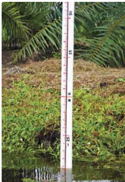
Figure 7-5: Water level gauge for water level monitoring in collection drain.
