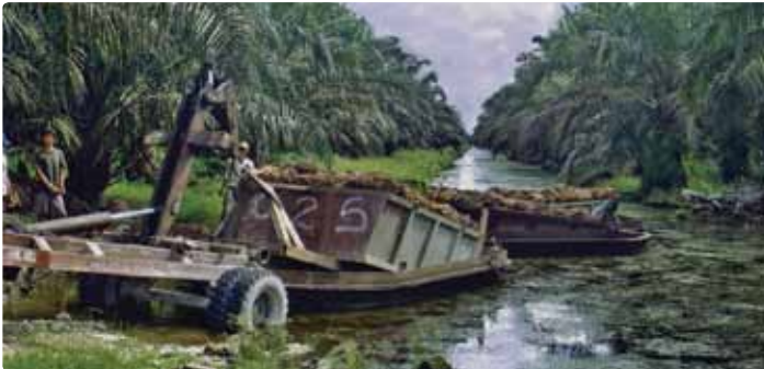
Figure 3-13: Following the contours and setting high water levels along collection drain in Woodman estate in Bintulu, Sarawak enables FFB to be transported by barge pulled by a small boat with a 15hp engine.
