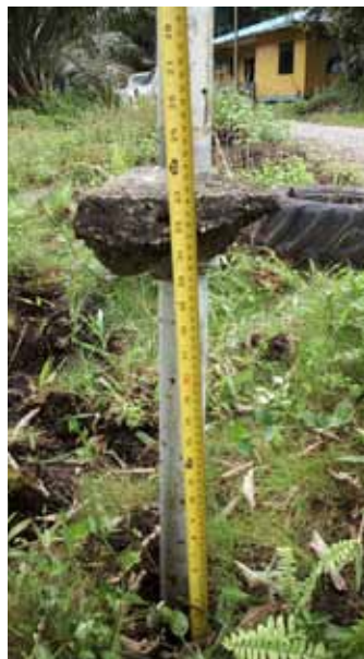
Figure 7-1: Example of subsidence pole installed together with a piezometer [Photograph on the left taken in 2011 and that on the right taken in 2018 for the same pole. Peat subsidence over time in this site is clearly visible.
