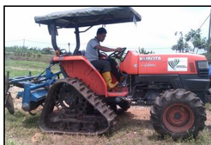
Tractors with large tracks to distribute weight over soft soil
